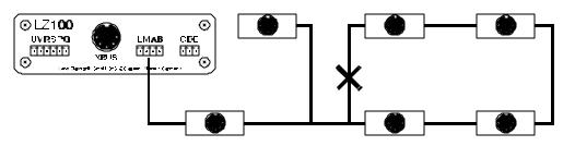
XpressNet devices can be powered directly from the XpressNet or powered through an external supply. The XpressNet device can be powered directly from the L and M 12 volts connections if the device draws less than 20mA when powered. This limit is to allow the bus to power multiple devices. If the devise requires more power than an external supply should be used.
